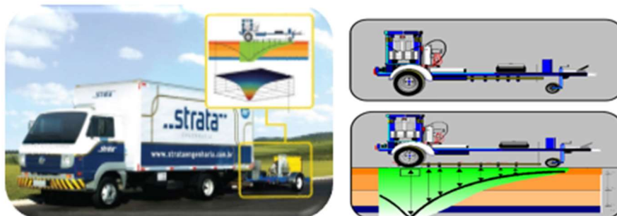
Figura 10: Falling Weight Deflectometer - FWD
