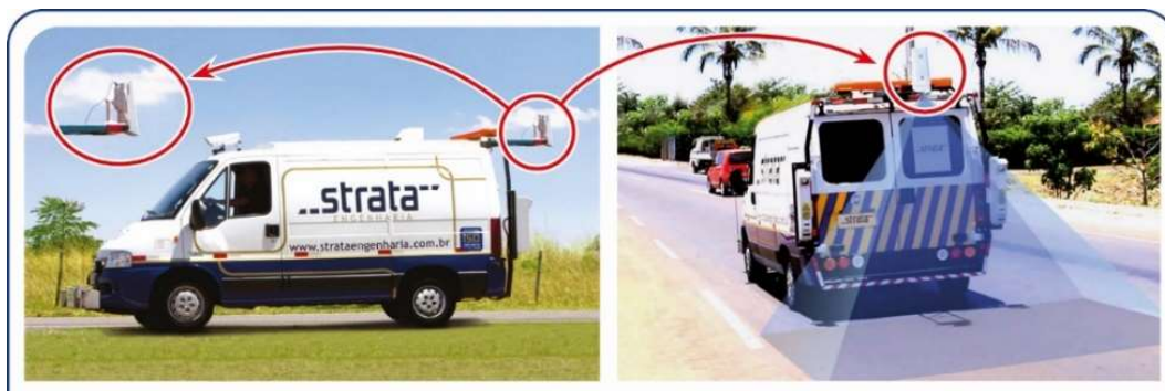
Figura 3: Detalhes do Orthogonal Pavement Recorder
