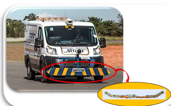
Figura 7: Road Surface Profilers Mark III
